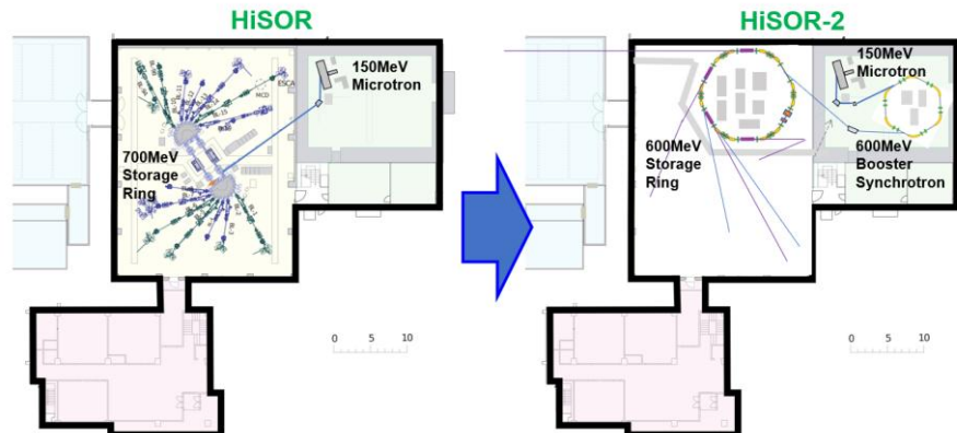
FIGURE 1. Layout of present HiSOR (left) and that of new HiSOR-2 (preliminary) (right).
