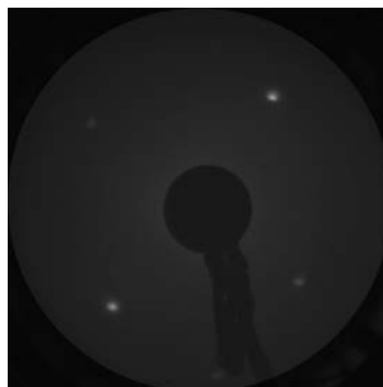
FIGURE 1. LEED image of the clean MnSi [001] surface which was obtained by mechanical polishing, and repeated Ar-ion sputtering and annealing in ultrahigh vacuum. The electron beam energy was E = 100 eV.
