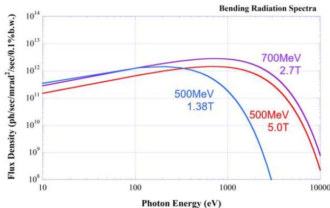
**FIGURE 1.** Synchrotron radiation spectra from bending magnets. That of the present HiSOR is 700MeV-2.7T. That of the new ring is 500MeV-5T (superconducting) and 500-1.38T (normal conducting).
