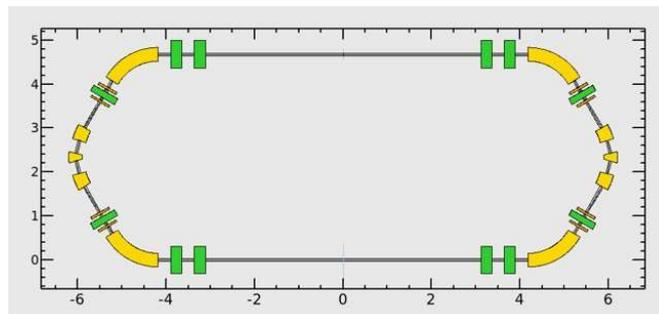
**FIGURE 1.** The layout of a compact storage ring with two superconducting bending magnets. The lattice consists of two triple-bend cells. The bending magnet of the center of the cells is hybrid, which consists of a superconducting bending magnet and two normal conducting bending magnets on both sides.
