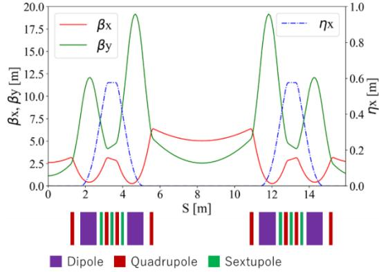
**FIGURE 2:** Betatron functions and dispersion function for one third of HiSOR-II storage ring [1].
