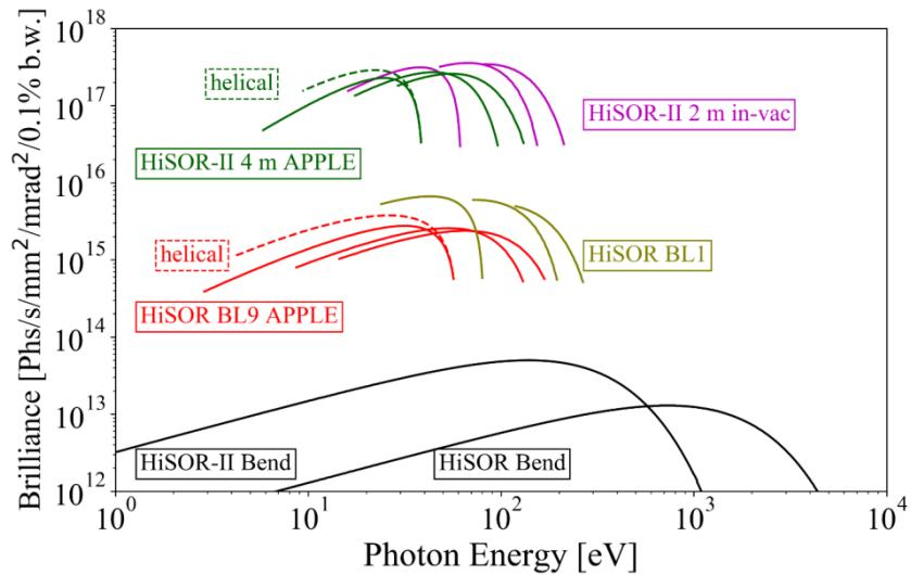
**FIGURE 3:** Comparison of brilliance of the synchrotron radiation from HiSOR and HiSOR-II.[1]
