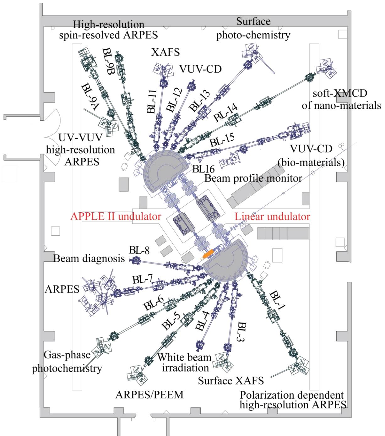
**Fig. 1:** Schematic view of the experimental hall.
