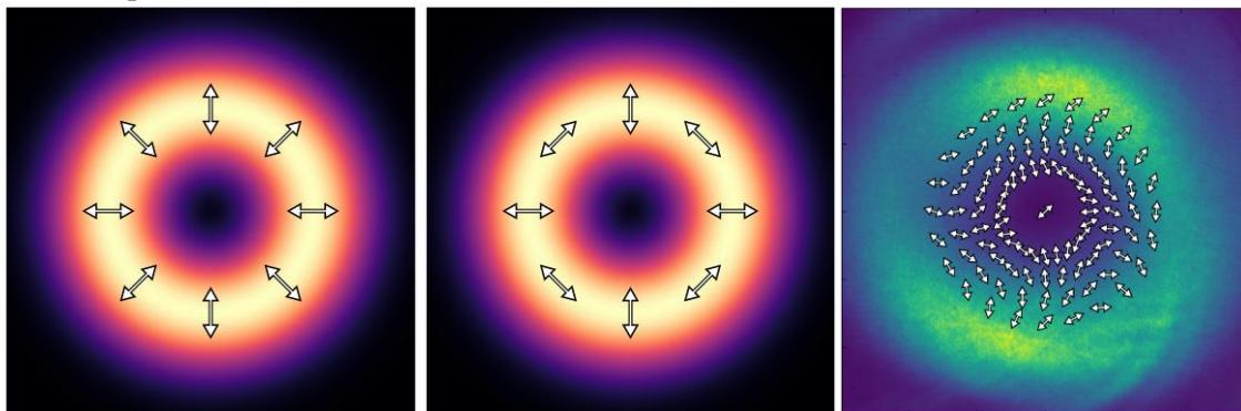
**Fig. 1.** A schematic illustration of vector beams (left and middle) and distributions of directions of polarization obtained by experiment (right). The arrows and back ground indicated polarization direction and intensity of each positions.
