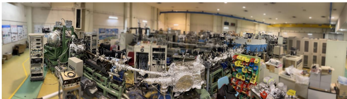
Figure 1. Beamline 1 (BL-1) (linear undulator beamline) for high-resolution angle-resolved photoemission spectroscopy (ARPES). The light polarization is changed by rotating the endstation ( s - and p -polarization are available).
